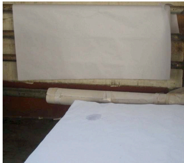
Amateur Hour at ONP. Note the water on the folding tables – and even on the paper being folded. Once paper is exposed to water, it is unsuitable for printing and loses strength.
